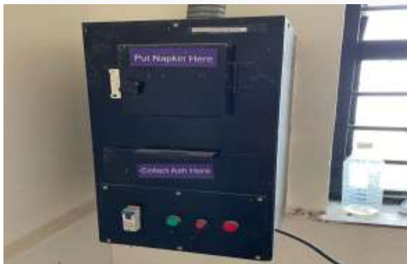
Sanitary Disposal Machine
